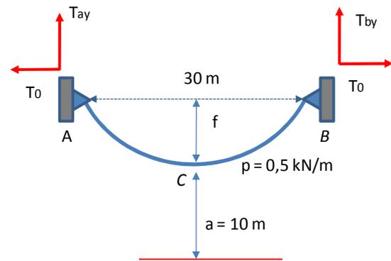
$$a = \frac{T_0}{p} \rightarrow T_0 = a \cdot p = 5 \text{ kN}$$
