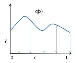
It is possible to calculate the resultant force and moment it creates just by integrating the curve, following the next process:
