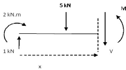
$$V_2 = 1 - 5 = -4 \text{ kN}$$
